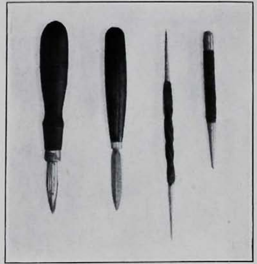
FIGURE 163 Burnisher Scraper Scratch Awl Center punch
