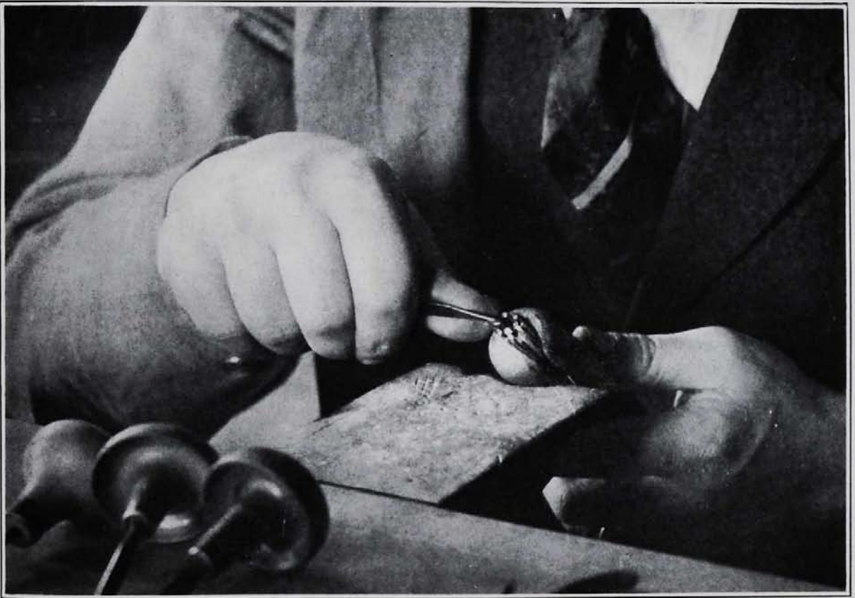
FIGURE 97. Bright cutting top and sides of prongs
