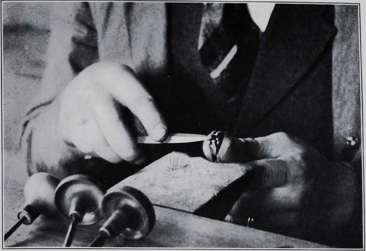
FIGURE 96. Filing the top of prongs
