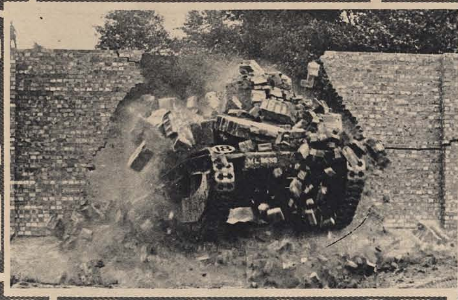
THE POWER OF THE MODERN TANK: A MEDIUM-SIZED TANK OF 1930 CRASHING THROUGH A NINE-INCH-THICK WALL OF BRICKS CEMENTED TOGETHER.
