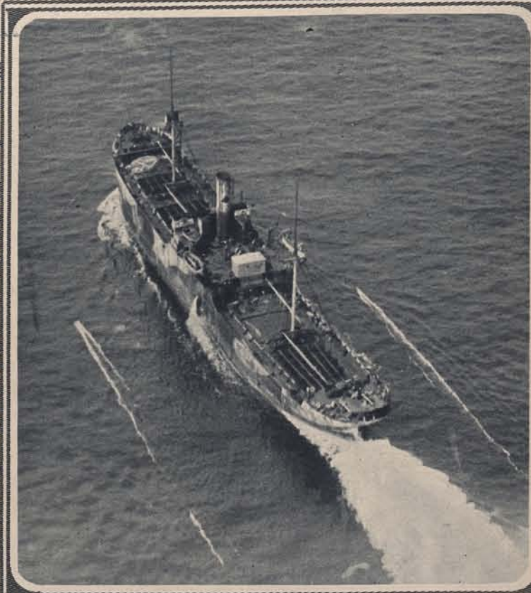
A SHIP PROTECTED FROM MINES BY PARAVANES, WHICH CUT THEM LOOSE. An effective device developed during the war was the protector paravane to guard a ship against moored mines. The paravane is towed on either side by means of a length of special wire. If the wire fouls the mooring wire of a mine, the mine is deflected away from the ship's path and is cut loose by the paravane.
