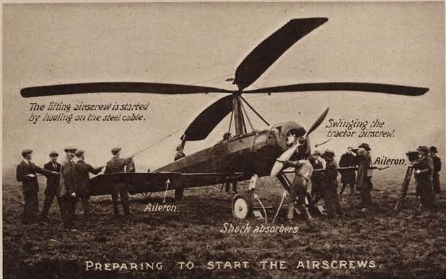
1925: THE COMING OF THE AUTOGIRO—A FLYING MACHINE ABLE TO HOVER IN THE AIR AND TO DESCEND VERTICALLY. On October 19, 1925, the Spanish engineer, Senor Juan de la Cierva, successfully demonstrated before Sir Samuel Hoare and the chief officers of the Air Ministry the autogiro machine which he had evolved after years of patient endeavour. Since that demonstration the inventor has much improved his designs, and autogiros, having proved their worth, are now in official use by the British Army.
