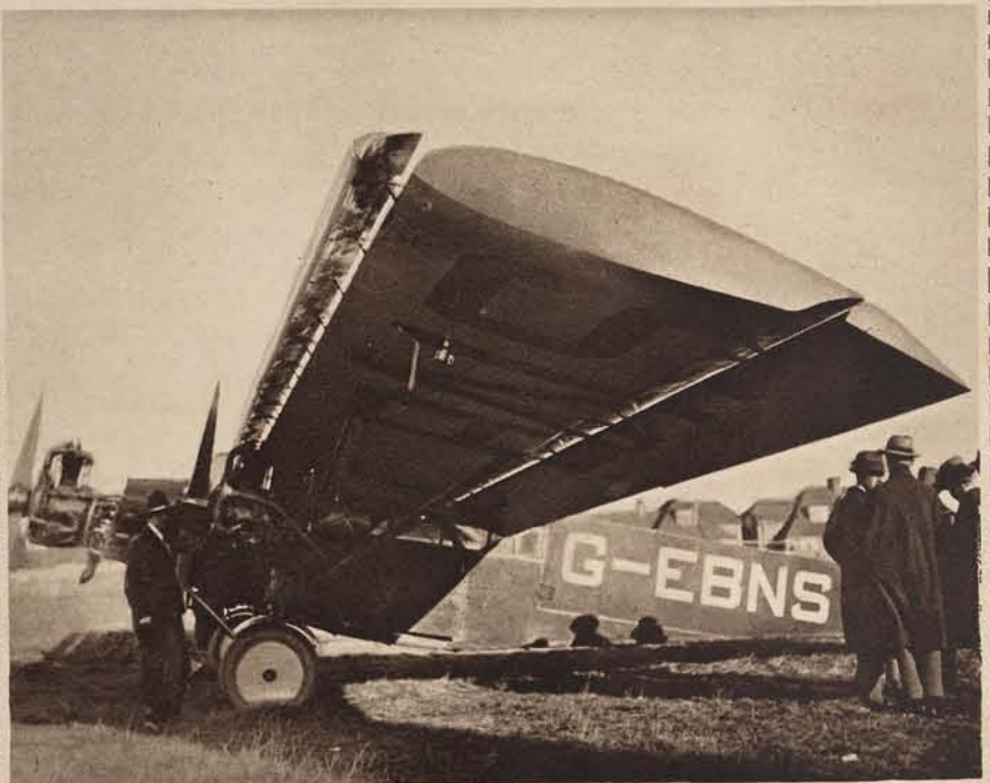
1926: THE SLOTTED WING—AN INVENTION OF OUTSTANDING IMPORTANCE IN REDUCING ACCIDENTS—A HANDLEY-PAGE AIR LINER SO EQUIPPED. The invention of an automatic slot fitted to the leading edge of the planes of aircraft—a British device which came into use in 1926—removed at once the principal cause of flying accidents. The slot eliminates the loss of control occurring when an aeroplane equipped with ordinary controls is "stalled," and so renders safe a much slower speed in the air. It has been of untold benefit to aviation.
