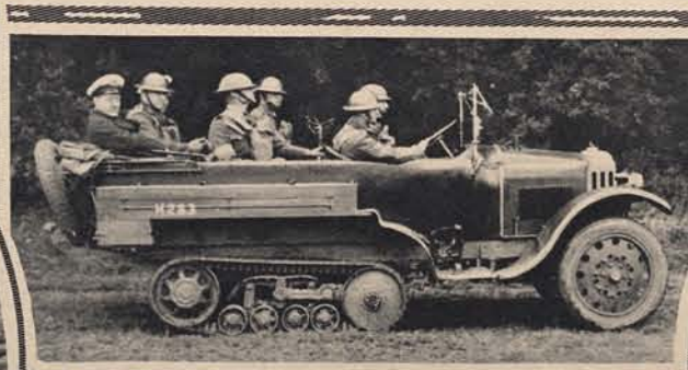
THE "HALF-TRACK CATERPILLAR" CAR: A PARTY OF OFFICERS TESTING ITS CROSS-COUNTRY CAPACITIES IN THE ARMY MANOEUVRES OF 1927.
