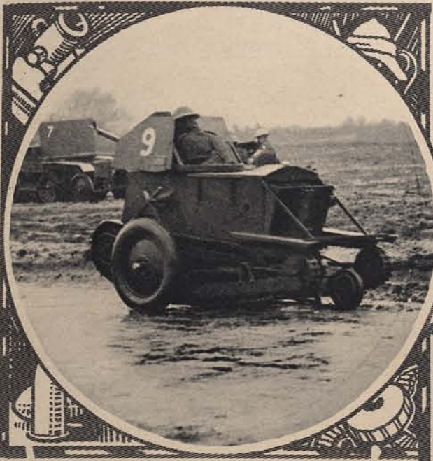
THE ONE-MAN TANK: A 1926 VERSION OF THE KNIGHT IN ARMOUR; ABLE TO TRAVEL AT A SPEED OF THIRTY MILES AN HOUR.
