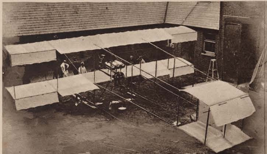
1910: MR. GRAHAME-WHITE'S FARMAN BIPLANE, IN WHICH HE ATTEMPTED A FLIGHT FROM LONDON TO MANCHESTER. This was the machine which Mr. Claude Grahame-White, one of the outstanding pioneers of British aviation, piloted with spectacular success in the summer of 1910. It was a Henry Farman biplane with a 50-h.p. Gnome rotary engine. On April 23 he had made a wonderful attempt to win the "Daily Mail" £10,000 prize for a flight from London to Manchester—won by M. Paulhan.
