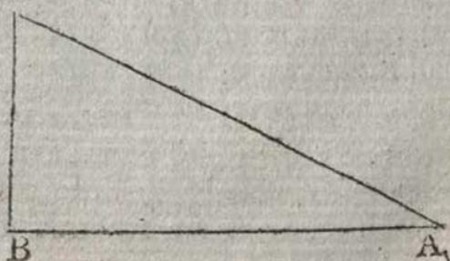
gave a line of 426 feet and seven inches from the centre of the pillar. At the extremity of the base A, a theodolite was placed, and previously being carefully adjusted, by putting the line of collimation in the telescope, parallel to the plane of the horizon, the angle B A C was observed to be twenty-nine degrees, thirty-nine minutes; thence the height of the *Cuttub Minar*, was found to be 242 feet and nearly six inches.
