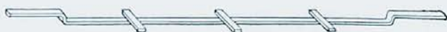
Strap-iron for arch, before bending. Its length depends on height and width of arch. Note cross-pieces
