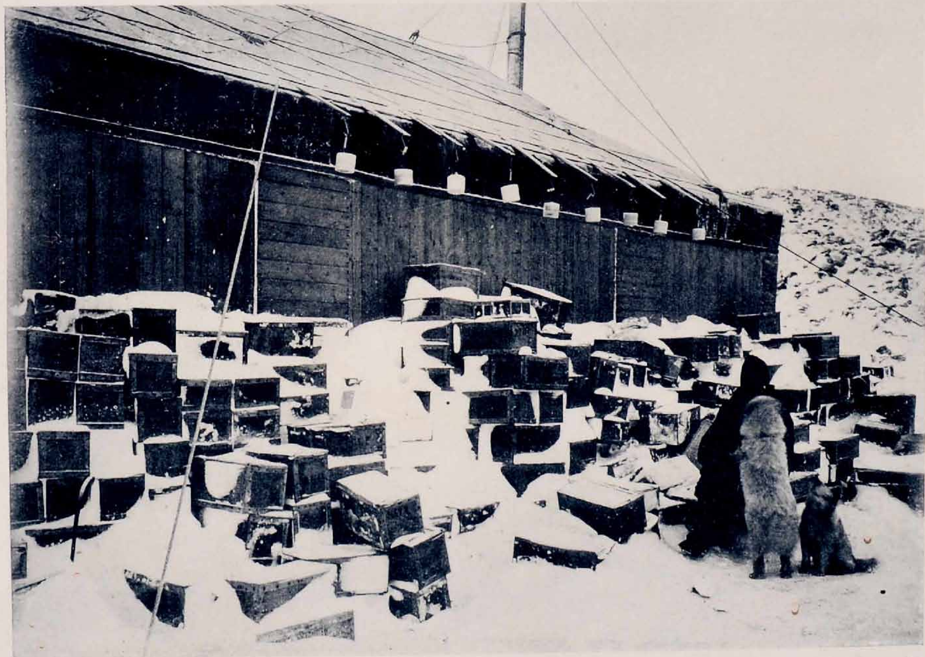
BLOCKS OF ICE HUNG IN THE WIND AT THE WINTER QUARTERS IN ORDER TO ASCERTAIN THE RATE OF EVAPORATION
