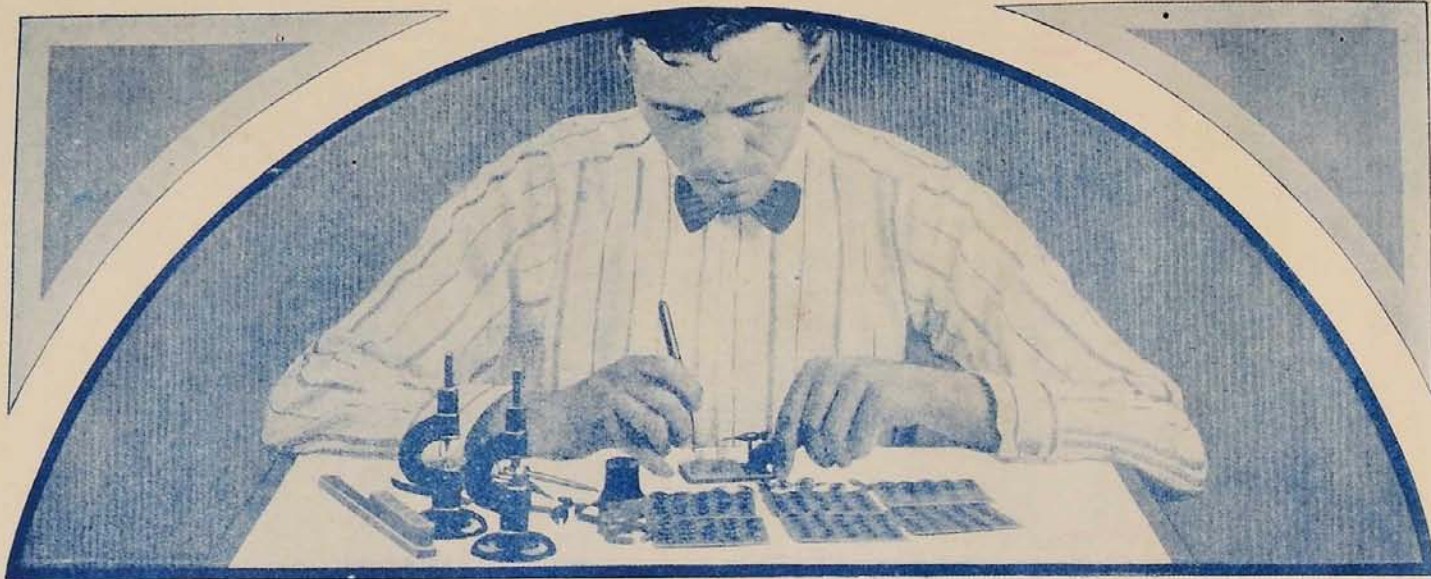
One of the inspections: Checking the balance, set in beat, against a master balance. The balances being tested are those of the Yankee, the lowest priced Ingersoll. This same method is used for the highest priced watches made.
