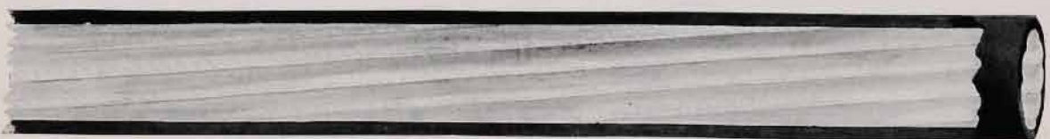
DIAGRAM SHOWING THE "RIFLING" OF A LEE-ENFIELD RIFLE.
