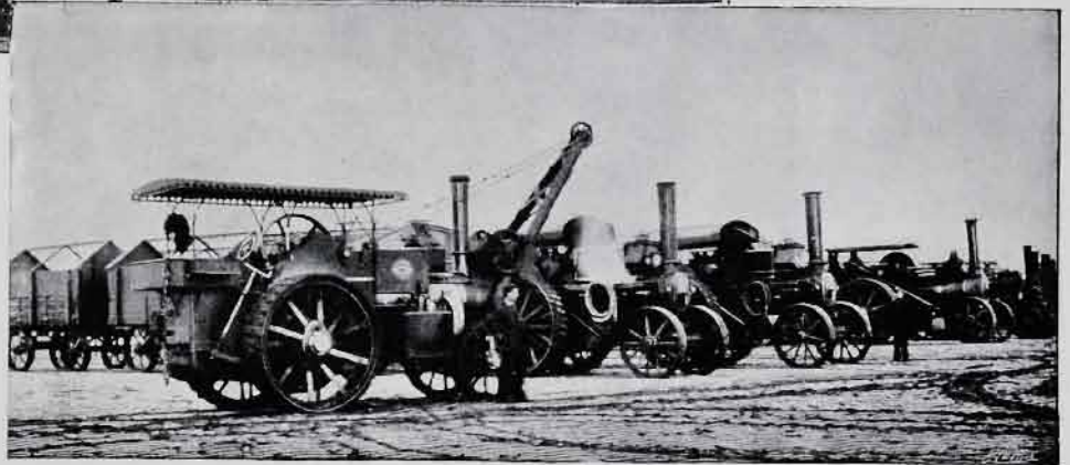
STEAM ROAD LOCOMOTIVES USED BY THE BRITISH GENERALS IN SOUTH AFRICA TO BRING UP SUPPLIES.
