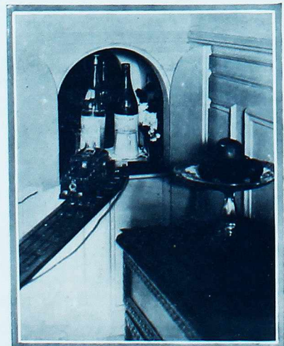
The Kitchen to Dining-room Electric Railway The train entering the dining-room
