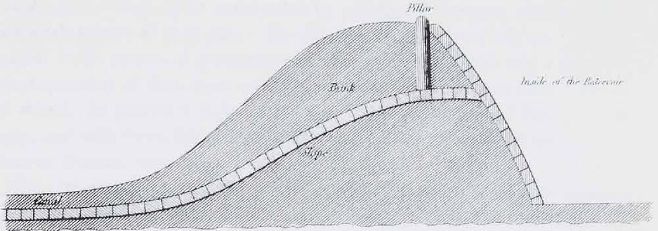
Transverse section of the bank and sluice of an Embankment Reservoir.
