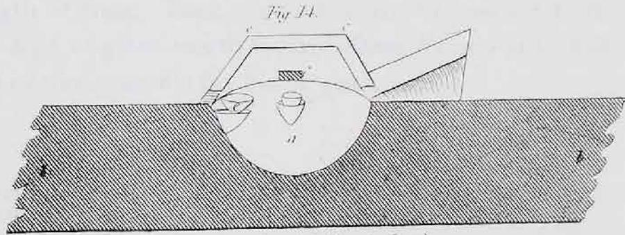
Vertical section of a glass-blower's fire-place.
