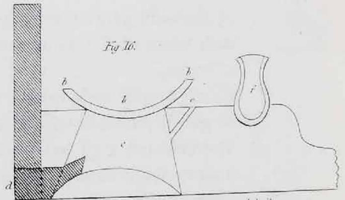
Vertical section of the furnace and boiler.
