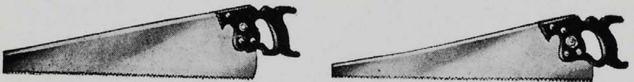
FIG. 2.15. Skewback and straight back saws.
