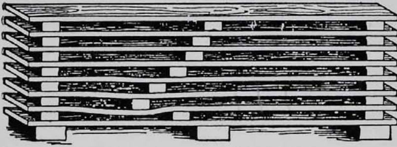
FIG. 2.106. Lumber carelessly supported.
