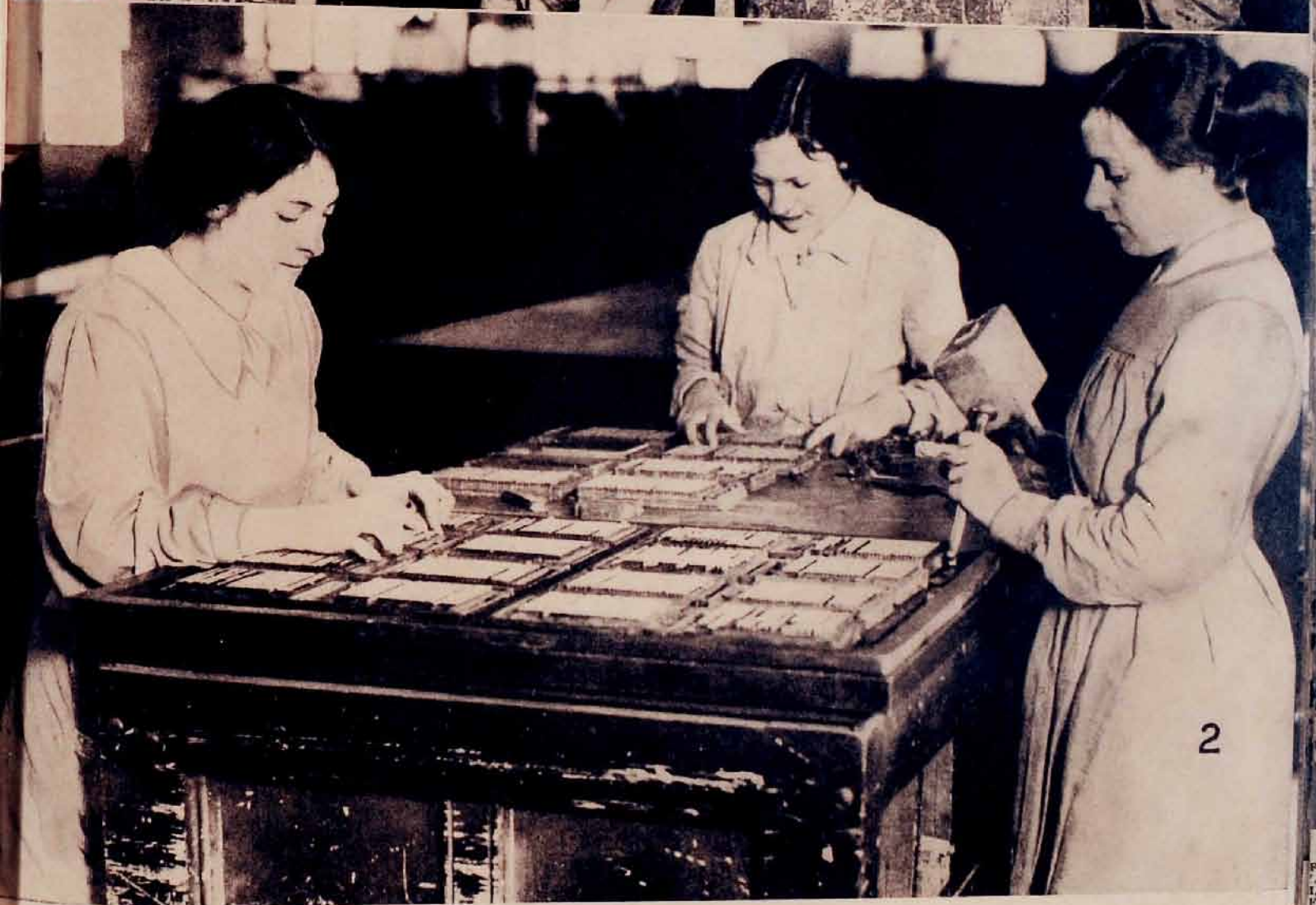
1.—MUNITION WORKERS WEARING RESPIRATORS WHILE FILLING SHELLS WITH TRINITROTOLUENE (T.N.T.), A HIGH EXPLOSIVE MUCH USED DURING THE WAR. 2.—WOMEN COMPOSITORS MAKING CORRECTIONS, ARRANGING COLUMNS OF TYPE AND LOCKING-UP PAGES PREPARATORY TO THEIR BEING CAST IN THE FOUNDRY BEFORE PRINTING. ALTHOUGH MADE OF METAL, THE TABLE AT WHICH THEY ARE WORKING IS CALLED A STONE.
