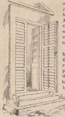
of each valve, and generally so ill-fitted, or so clogged with paint, as to leave wide interstices for the admittance of the rain and dust. Against these evils, our only protection is the folding glass doors that you may observe within the venetians, though, as I have already stated, the rain is often but turned in its course to flow in, from beneath, upon the mat.
